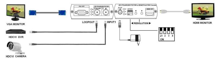
\* 3 outputs: HDMI, VGA, loop output as a distributor.
